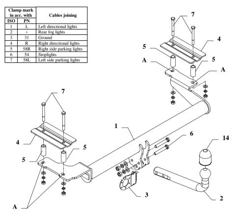
This towing hitch is designed to assembly in following cars: **FORD ESCORT IV 3/5 doors,** produced since 01.1996 till 1998, catalogue no. **C10** and is prepared to tow trailers max total weight **1250 kg** and max vertical load **50 kg**.
