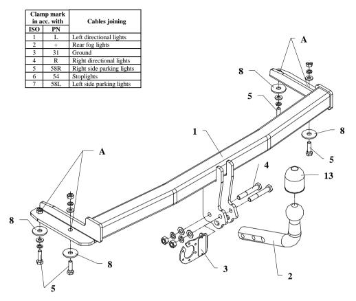
This towbar is designed to assembly in following cars: SEAT IBIZA 4-5 doors GLX/GTI produced since 02.1996 till 08.1999, catalogue no. SC07 and is prepared to tow trailers max total weight 1100 kg and max vertical load 50 kg.
