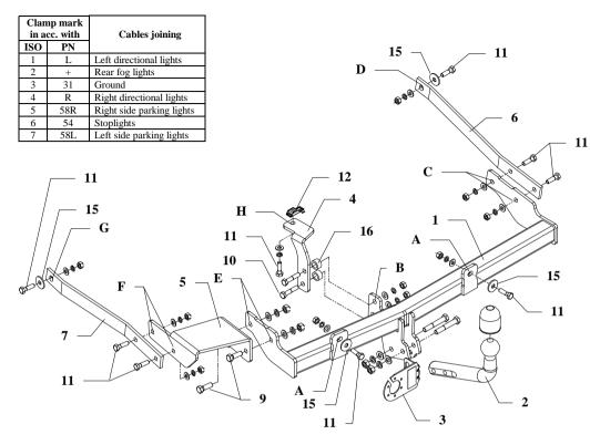
This towbar is designed to assembly in following cars: CITROEN XANTIA ESTATE produced since 1995 till 2000, catalogue no. P17 and is prepared to tow trailers max total weight 1500 kg and max vertical load 85 kg.
