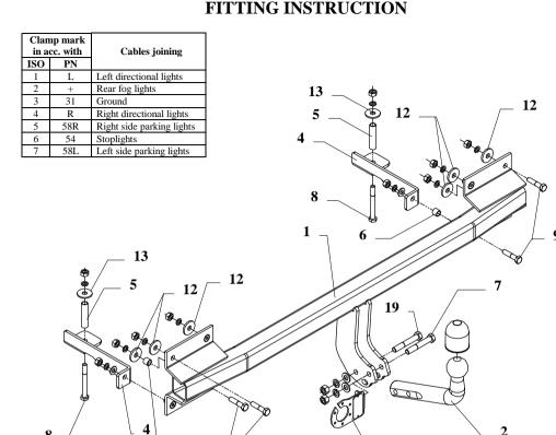
This towing hitch is designed to assembly in following car: **KIA SEPHIA 4/5 door**, produced since 01.1993 till 1998, catalogue no. **T44** and is prepared to tow trailers max total weight **1450 kg** and max vertical load **50 kg**.
