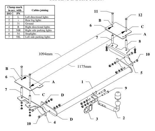
This towing hitch is designed to assembly in following cars: FIAT PALIO WEEKEND ESTATE, produced since 1998 till 2001, catalogue no. R15 and is prepared to tow trailers max total weight 1200 kg and max vertical mass 70 kg.
