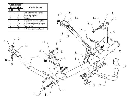
This towbar is designed to assembly in following cars: PEUGEOT 806 (5 doors and VAN) and EXPERT (metal built-up), CITROEN EVASION (5 doors and VAN) and JUMPY (metal built-up), FIAT ULYSSE (5 doors and VAN) and SCUDO (metal built-up), LANCIA Z (5 doors and VAN), all produced since 1994 till 12.2006, catalogue number R17 and is prepared to tow trailers max total weight 1800 kg and max vertical mass 80 kg.
