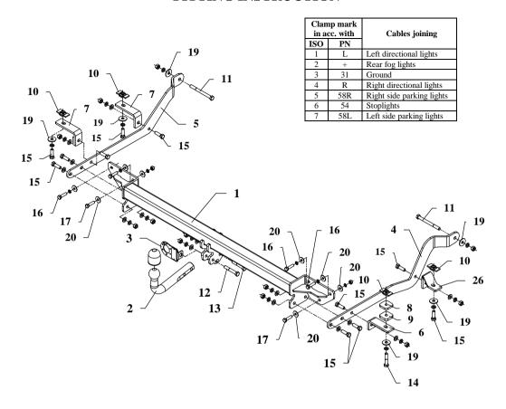
This towing hitch is designed to assembly in following cars: **FIAT DUCATO L4, PEUGEOT BOXER L4, CITROEN JUMPER L4, metal built-up,** produced since 2006, catalogue no. **R42** and is prepared to tow trailers max total weight up to **3100 kg** and max vertical load **124 kg**.
