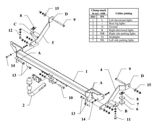
This towbar is designed to assembly in following cars: FIAT DUCATO (L1, L2, L3), PEUGEOT BOXER (L1, L2, L3), CITROEN JUMPER (L1, L2, L3), metal built-up, produced since 2006, catalogue no. R39 and is prepared to tow trailers max total weight 2500 kg and max vertical load 120 kg.
