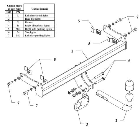
This towbar is designed to assembly in following car: **SKODA FELICIA PICK UP**, produced since 1996, catalogue no. **H11** and is prepared to tow trailers max total weight **1000 kg** and max vertical mass **50 kg**.
