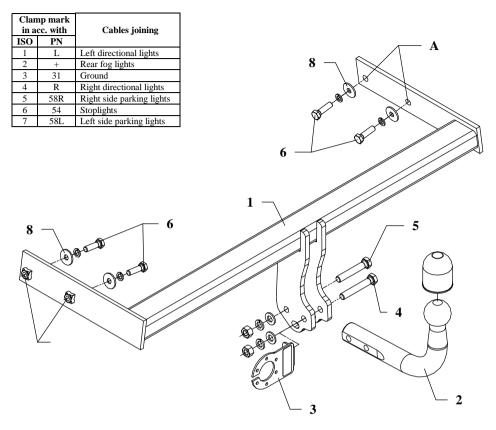
This towing hitch is designed to assembly in following cars: **VOLVO S80 (4 doors)** and **V70 (estate)**, produced since 08.2006, catalogue no. **L20** and is prepared to tow trailers max total weight **2100 kg** and max vertical cup load **90 kg**.
