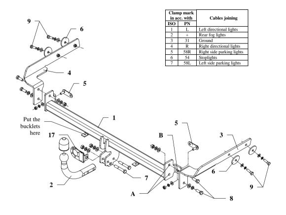
This towbar is designed to assembly in following cars: **FORD FOCUS ESTATE**, produced since 1998 till 2005, catalogue no. **C29** and is prepared to tow trailers max total weight **1400 kg** and max vertical load **75 kg**.
