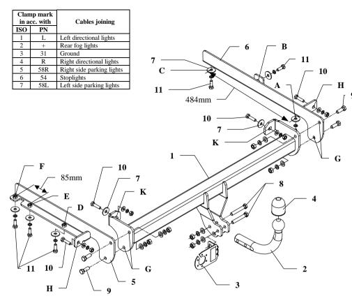
This towing hitch is designed to assembly in following cars: **HONDA CIVIC ESTATE**, produced since 1997 till 10.2000, catalogue no. **Y05** and is prepared to tow trailers max total weight up to **1300 kg** and max vertical mass **50 kg**.
