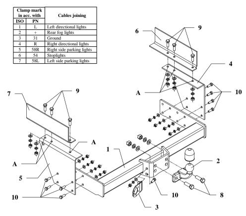
This towbar is designed to assembly in following cars: **FIAT IVECO DAILY metal build-up, loading platform,** produced since 1989 till 04.1999, catalogue number **R13** and is prepared to tow trailers max total weight **3000 kg** and max vertical load **100 kg**.
