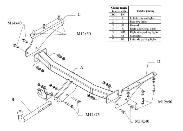
This towing hitch is designed to instalment in following car: **JEEP CHEROKEE (KJ)**, catalogue no. **JP02**, produced since 09.2001 till 2007 and is prepared to tow trailers max total weight up to **3500 kg** and max vertical mass **100 kg**.
