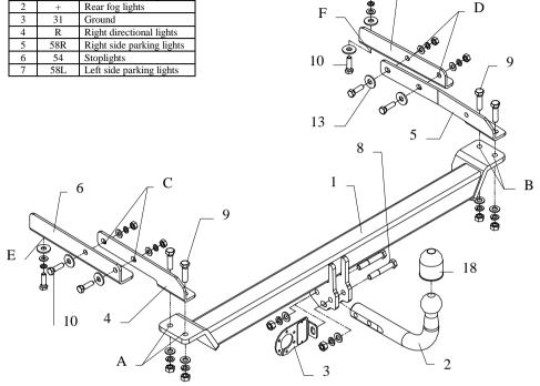
This towbar is designed to assembly in following cars: MERCEDES C208, W202, S202, C Class, CLK, 4 door, ESTATE, produced since 11.1993 till 05.2002, catalogue no. D14 and is prepared to tow trailers max total weight 1800 kg and max vertical mass 75 kg.
