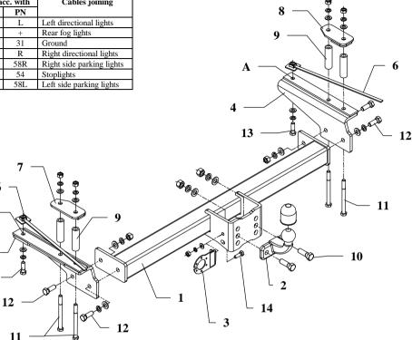
This towbar is designed to assembly in following cars: NISSAN PATROL GR (Y60), produced since 01.1989 till 12.1997, catalogue no. V09 and is prepared to tow trailers max total weight 3000 kg and max vertical load 100 kg.
