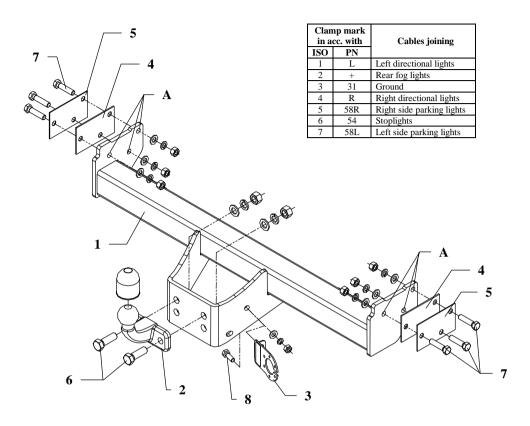
This towing hitch is designed to assembly in following cars: **NISSAN TERRANO II, 3/5 door,** produced since 1993 till 2003, **FORD MAVERICK, 3/5 door,** produced since 1993 till 2001 catalogue no. **V18** and is prepared to tow trailers max total weight **3000 kg** and max vertical mass **100 kg**.
