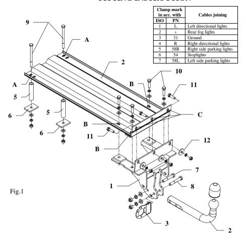
This towbar is designed to assembly in following car: **OPEL OMEGA** "A" **4 doors**, produced since 1986 till 1993, catalogue number **E14** and is prepared to tow trailers max total weight **1850 kg** and max vertical load **75 kg**.
