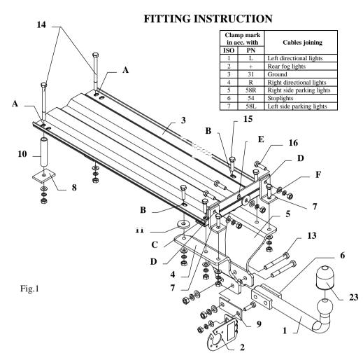
This towbar is designed to assembly in following car: **OPEL OMEGA**,,**B**" **4 doors**, produced since 04.1994, catalogue no. **E16** and is prepared to tow trailers max total weight **2100 kg** and max vertical load **75 kg**.
