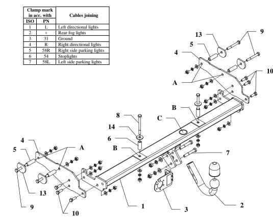
This towing hitch is designed to assembly in following car: CITROEN C15, produced since 1985 till 2007, catalogue no. P06 and is prepared to tow trailers max total weight 900 kg and max vertical load 45 kg.
