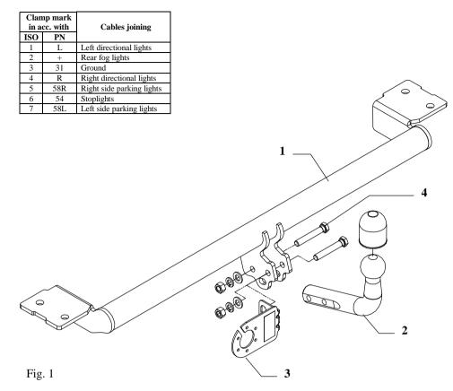
This towbar is designed to assembly in following car: **TOYOTA AVENSIS 4-5 doors,** produced since 1997 till 12.2002, catalogue no. **O05**, and is prepared to tow trailers max total weight **1400 kg** and max vertical load **75 kg**.
