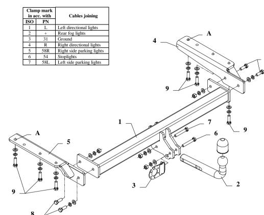
This towbar is designed to assembly in following cars: **TOYOTA LANDCRUISER J90/J95, 3 door,** produced since 1996 till 12.2002, catalogue no. **O45** and is prepared to tow trailers max total weight **2800 kg** and max vertical load **130 kg**.
