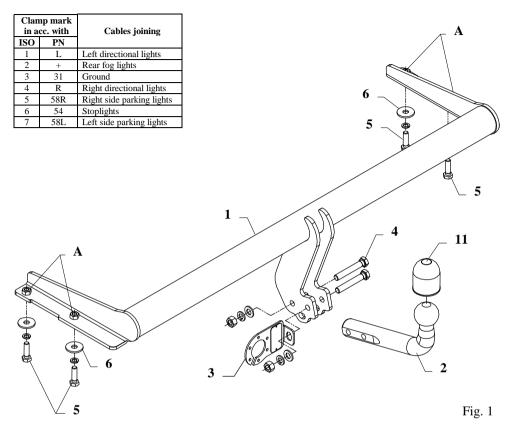
This towing hitch is designed to assembly in following car: VOLKSWAGEN GOLF III, produced since 11.1991 till 1997, catalogue no. K05 and is prepared to tow trailers max total weight 1500 kg and max vertical load 75 kg.
