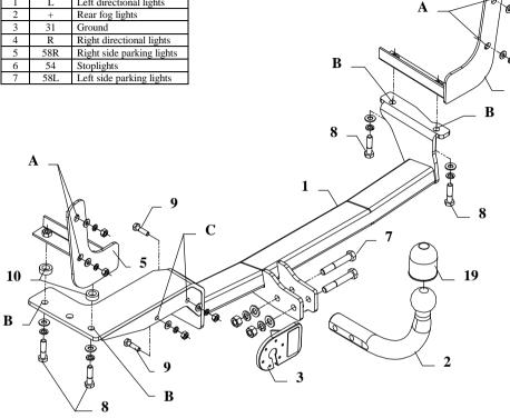
This towbar is designed to assembly in following car: VOLKSWAGEN POLO 3/5 doors, produced since 09.1994 till 09.1999, catalogue no. K21 and is prepared to tow trailers max total weight 1200 kg and max vertical load 50 kg.
