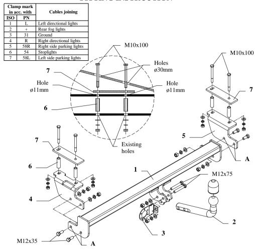
This towbar is designed to assembly in following cars: **DAEWOO NEXIA, 3-5 door,** produced since 1995 till 1997, catalogue no. **X02** and is prepared to tow trailers max total weight **1200 kg** and max vertical load **70 kg**.
