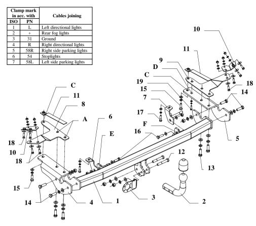
This towing hitch is designed to assembly in following car: **TOYOTA COROLLA VERSO**, produced since 04.2004 till 2007, catalogue no. **O59** and is prepared to tow trailers max total weight **1450 kg** and max vertical load **52 kg**.
