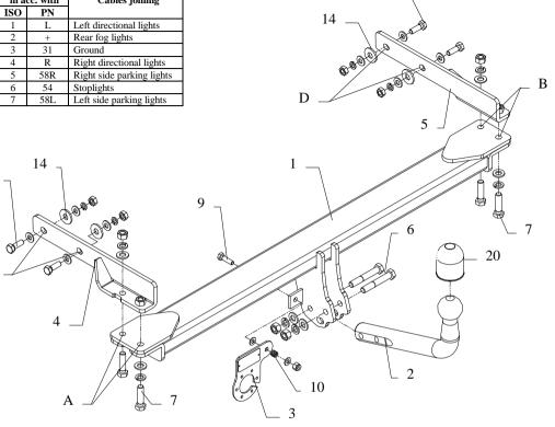
This towing hitch is designed to assembly in following cars: MERCEDES S210 CLASS E, ESTATE, produced since 1996 till 03.2002, catalogue no. D31 and is prepared to tow trailers max total weight 2300 kg and max vertical load 85 kg.
