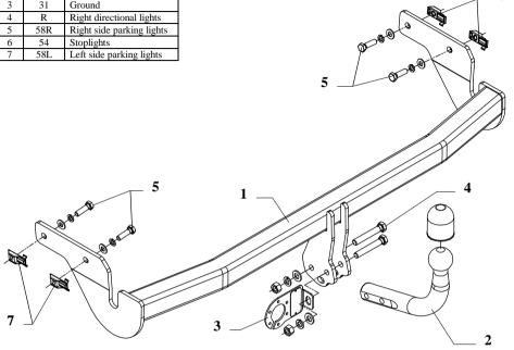
This towbar is designed to assembly in following car: PEUGEOT 207, produced since 2006, catalogue number F30 and is prepared to tow trailers max total weight 1150 kg and max vertical load 46 kg.
