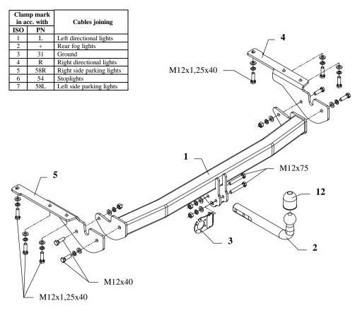
This towbar is designed to assembly in following cars: **TOYOTA RAV-4 "X", model without the spare wheel,** produced since 2005, catalogue no. **O66** and is prepared to tow trailers max total weight **2000 kg** and max vertical load **75 kg**.
